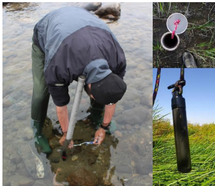
Figure 13 - Installation of water level loggers outside piezometers for measuring river water level (left) and inside pipe for measuring groundwater level (right).
