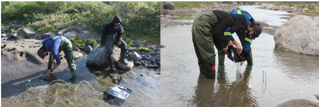
Figure 8 - Installed seepage meter at the bottom of the river (left), measuring the collected water at the end of the day (right).
