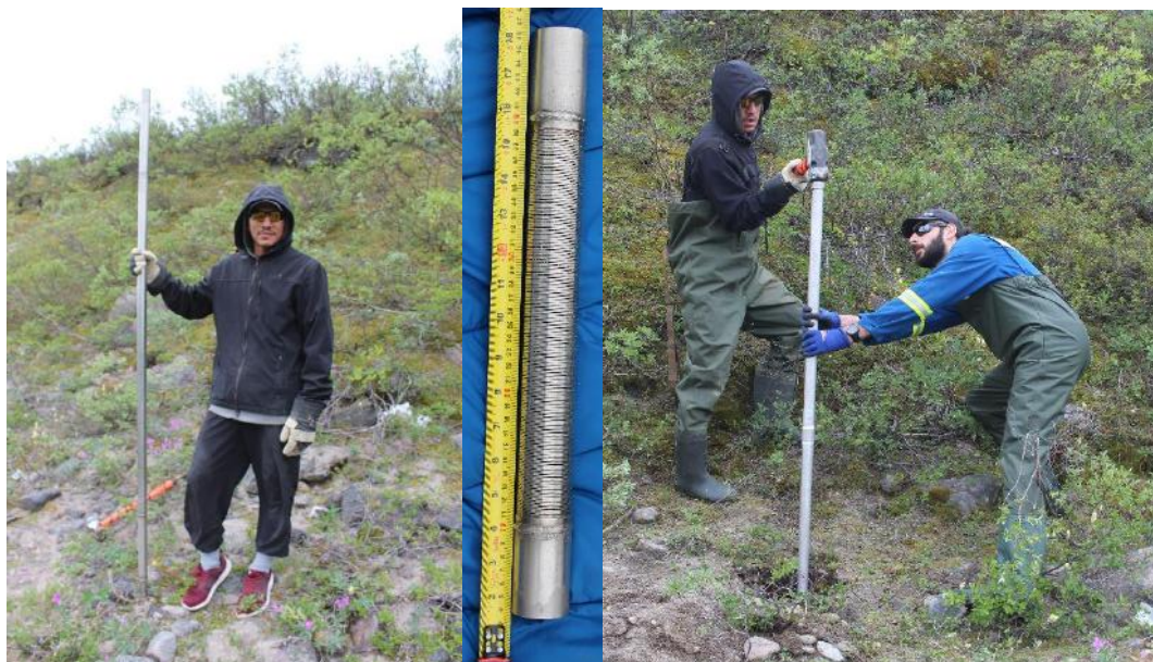
Figure 10 - One stainless steel pipe (left), piezometer screen (middle) and piezometer installation.
